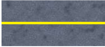
Continuous Longitudinal Line along the Carriageway
